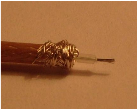
Fig. 26: Prepared Coax Cable
