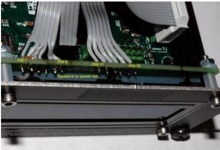
Fig. 17: Solder Ribbon Cable
