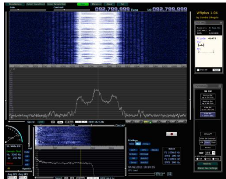
Fig. 124: FM Reception with a 48 kHz card
