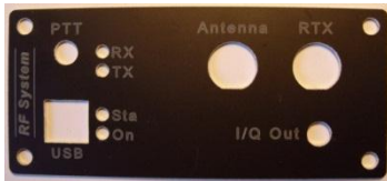
Fig. 21: Type 2 Rear Panel; In this case, do not install the antenna jack on the PMSDR circuit board!
